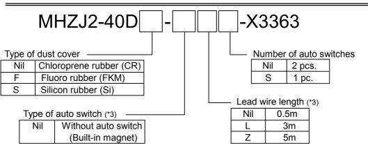
\*3) Types of applicable auto switches are the same as standard MHZJ2 Series (with dust cover). Note: Switch types D-Y5/6 and D-Y7 which can be mounted on Ø40mm of standard MHZ2 Series, cannot be mounted when equipped with dust cover. (Water resistant solid state switch D-F9BAL can be mounted.)
