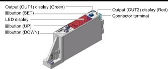
Output (OUT1) display (Green): LED is ON when the switch output (OUT1) is
