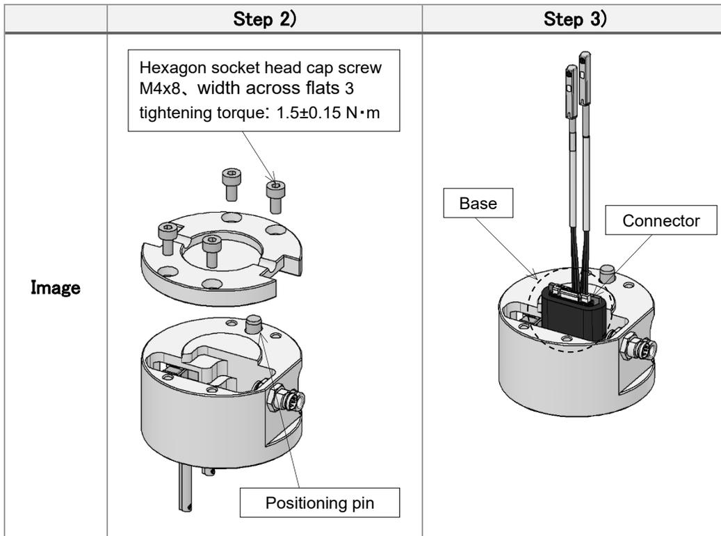
\*Figure shows the mounting interface, manual type.
