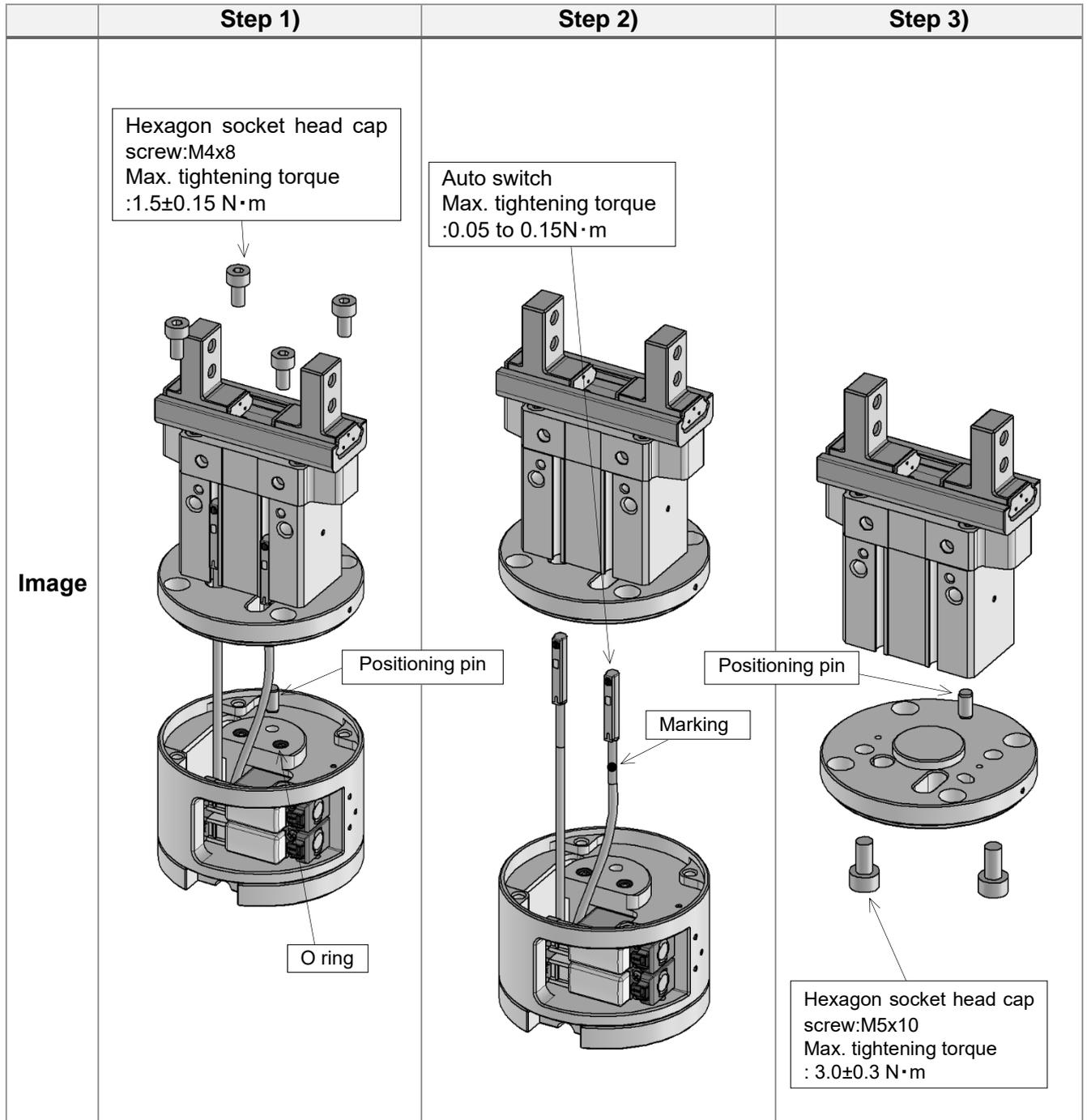
\*Figure shows the mounting interface, manual type.
