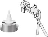
2. Tighten the nut until it touches the end surface of the body, and then tighten it an additional 1/8 turn. If the nut won't turn any further, then it means a sufficient tightening has occurred. Refer to the proper tightening torques shown below.
