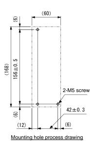
Mounting screw Screw size:M5 Tightening torque:3.24[N⋅m]
