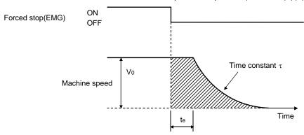
Fig. 12.3 Dynamic brake operation diagram
