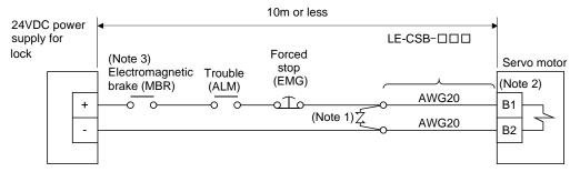
Note 1. Connect a surge absorber as close to the servo motor as possible.
