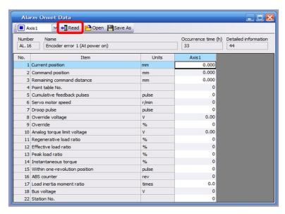
Click the "Read" button to read the monitor data at error occurrence from the driver. Read results are displayed as follows.
