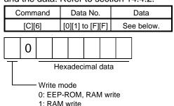
When the speed data is changed frequently through communication, set "1" to the write mode to change only the RAM data in the driver. When changing data frequently (once or more within one hour), do not write it to the EEP-ROM.
