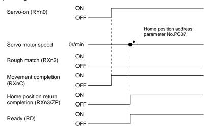
The parameter No.PC07 (home position return position data) setting value is the positioning address after the home position return is completed.
