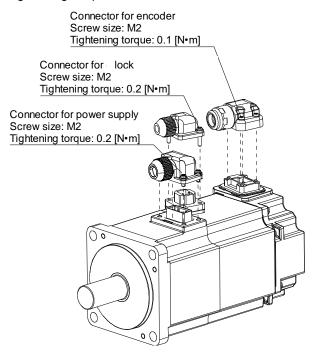
(3) The servo motor fitting part of each connector is provided with a splash-proof seal (O ring). When mounting a connector, use care to prevent the seal (O ring) from dropping and being pinched. If the seal (O ring) has dropped or is pinched, a splash-proof effect is not produced.
