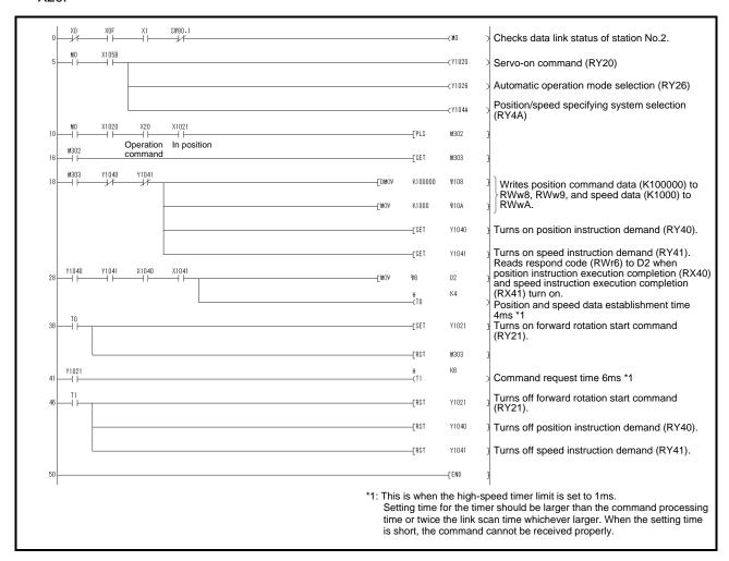
(3) Remote register-based point table No. setting (incremental value command system)
