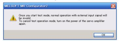
Click the "OK" button to display the setting screen of the DO forced output.
