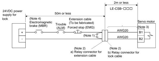
Note 1. Connect a surge absorber as close to the servo motor as possible.
