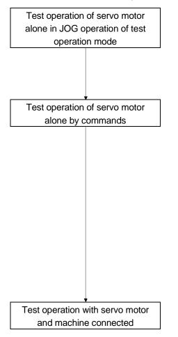
In this step, confirm that the driver and servo motor operate normally.
