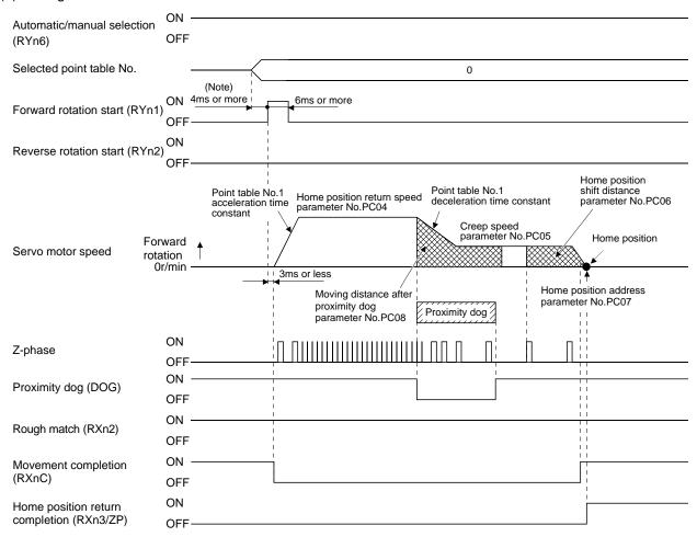
Note. Configure a sequence that changes the point table selection earlier, considering the delay time of CC-Link communication.
