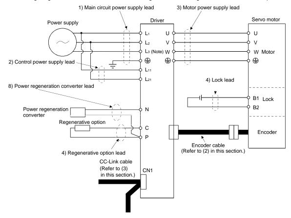
Use the 600 V Grade heat-resistant polyvinyl chloride insulated wire (HIV wire) for wiring. The following shows the wire size selection example.
