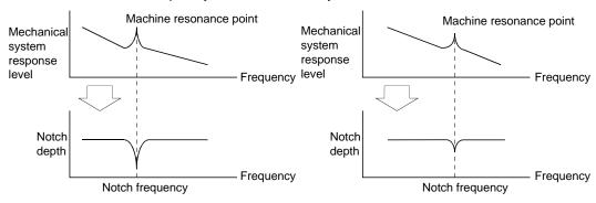
When machine resonance is large and frequency is low When machine resonance is small and frequency is high
