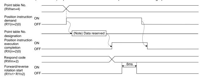
Note. This data is stored into RAM of the driver. Hence, the data is cleared when power is switched off.
