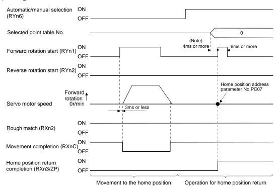
Note. Configure a sequence that changes the point table selection earlier, considering the delay time of CC-Link communication.
