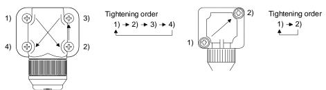
Connector for power supply, connector for encoder
