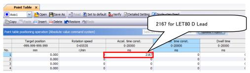
\*5 : Use the acceleration time constant of Point table No.1 as the acceleration time constant (msec) of Home position return. Set the recommended value in the above figure.
