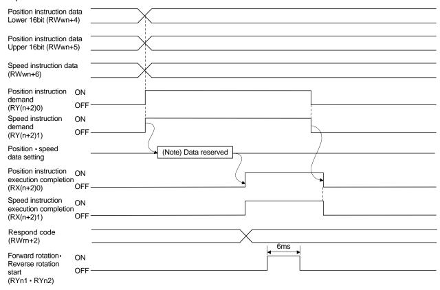
Note. This data is stored into RAM of the driver. Hence, the data is cleared when power is switched off.
