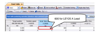
\*5. Use the acceleration time constant of Point table No.1 as the acceleration time constant (msec) of Home position return. Set the recommended value in the above figure. Refer to "LECSC2-T□ Operation Manual ", section 5.4.2 for how to set the Point table.
