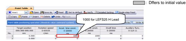
\*5. Use the acceleration time constant of Point table No.1 as the acceleration time constant (msec) of Home position return. Set the recommended value in the above figure. Refer to "LECSC2-T□ Operation Manual ", section 5.4.2 for how to set the Point table.
