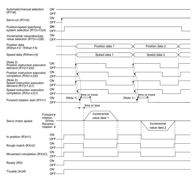
Note 1. Configure a sequence that changes the point table selection earlier, considering the delay time of CC-Link communication.
