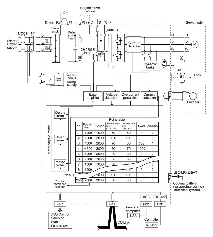
Note 1. The built-in regenerative resistor is not provided for the LECSC2-T5.
