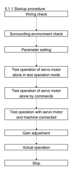
Check whether the driver and servo motor are wired correctly using visual inspection, DO forced output function (Section 7.7.4), etc. (Refer to section 5.1.2.)
