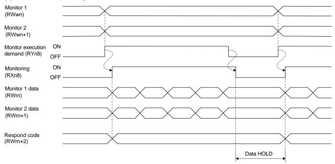
Set the monitor codes No. (0000 to 001D) (refer to section 3.5.3) to Monitor 1 (RWwn) and Monitor 2 (RWwn+1) and turn Monitor output execution demand (RYn8) to ON. Turning Monitor execution demand (RYn8) to ON sets the next data. Data are all hexadecimal numbers. At this time, Monitoring (RXn8) turns to ON at the same time.
