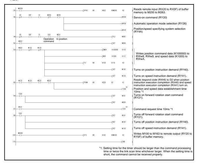
(3) Remote register-based point table No. setting (incremental value command system)
