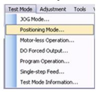
Click "Positioning Mode" on the menu bar and click "Move Distance Unit Selectiom" on the menu. Check Command pulse unit (Electronic gear valid) and click OK. Electronic gear ratio that is set in the PA05 / PA06 / PA07 is enabled.
