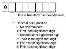
By way of example, here is described how to process the set data when a value of "15.5" is sent.
