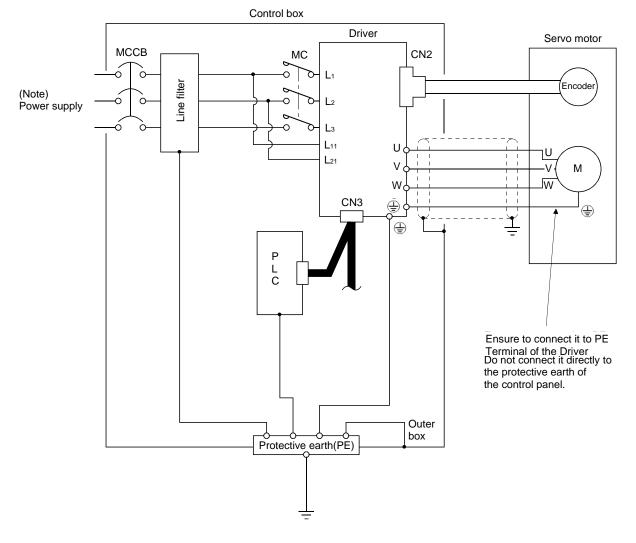
Note. For 1-phase 200 to 230VAC or 1-phase 100 to 120VAC, connect the power supply to  $L_1 \cdot L_2$  and leave  $L_3$  open. There is no  $L_3$  for 1-phase 100 to 120VAC power supply. Refer to section 1.2 for the power supply specification.
