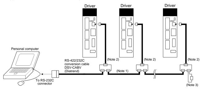
Note 1. Refer to section 141 for cable wiring.
