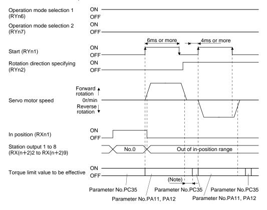
Note. Torque limit delay time can be set in the parameter No.PD26.
