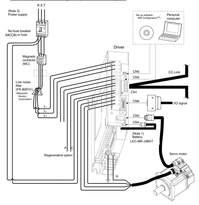
Note 1. The battery is used for the absolute position detection system in the position control mode.
