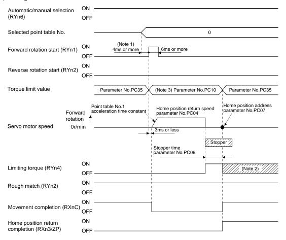
Note 1. Configure a sequence that changes the point table selection earlier, considering the delay time of CC-Link communication.
