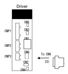
● Direct connection type(cable length 10m or less, IP65)
