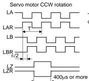
Time cycle (T) is determined by the settings of parameter No.PA15 and PC19.
