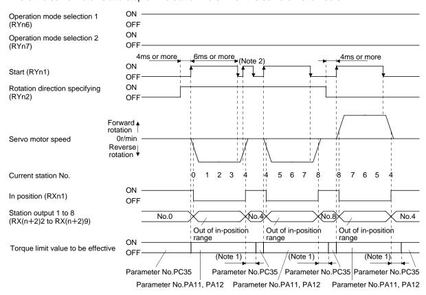
Note 1. Torque limit delay time can be set in the parameter No.PD26.
