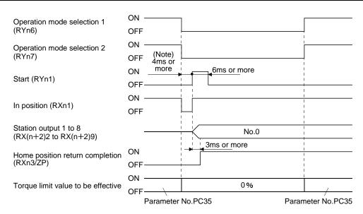
Note. Configure a sequence that changes the operation mode earlier, considering the delay time of CC-Link communication.
