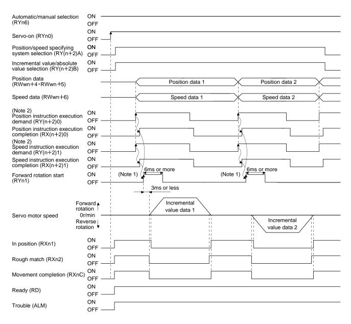
Note 1. Configure a sequence that changes the point table selection earlier, considering the delay time of CC-Link communication.
