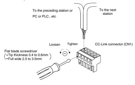
Use of a flat-blade torque screwdriver is recommended to manage the screw tightening torque. The following table indicates the recommended products of the torque screwdriver for tightening torque management and the flat-blade bit for torque screwdriver. When managing torque with a Phillips bit, please consult us.
