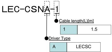
\*LEC-CSNA-1 is 10126-3000PE(Connector)/10326-52F0-008(Shell kit) of Sumitomo 3M Limited or equivalent goods.
