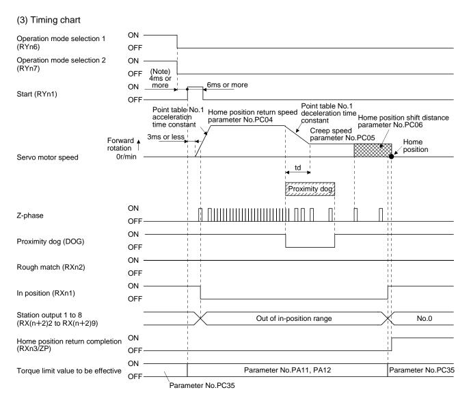
Note. Configure a sequence that changes the operation mode earlier, considering the delay time of CC-Link communication.
