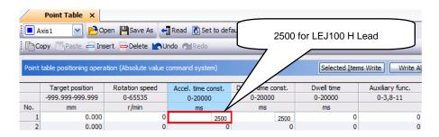
\*5. Use the acceleration time constant of Point table No.1 as the acceleration time constant (msec) of Home position return. Set the recommended value in the above figure. Refer to "LECSC2-T□ Operation Manual ", section 5.4.2 for how to set the Point table.
