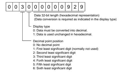
Since the display type is "0" in this case, the hexadecimal data is converted into decimal.  $00000929H\rightarrow2345$
