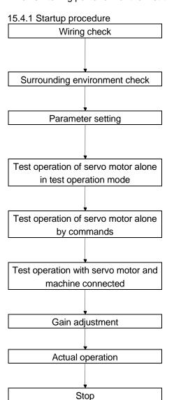
Check whether the driver and servo motor are wired correctly using visual inspection, DO forced output function (Section 7.7.4,), etc. (Refer to section 15.4.3.)
