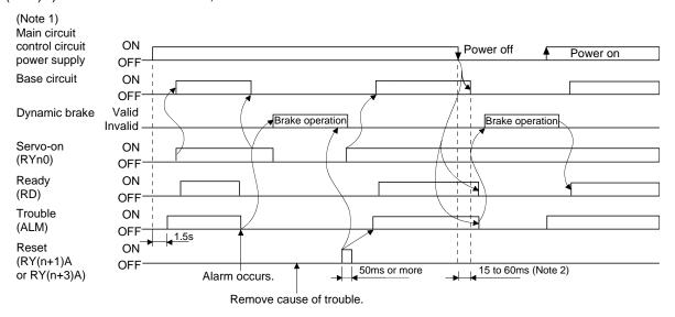
Note 1. Shut off the main circuit power as soon as an alarm occurs.
