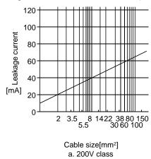
Fig. 13.4 Leakage current example (lg1, lg2) for CV cable run in metal conduit
