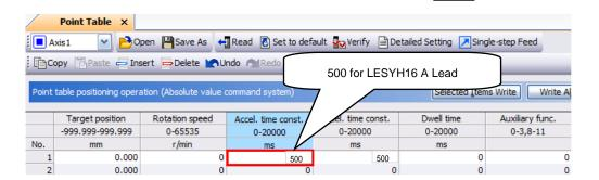
\*5. Use the acceleration time constant of Point table No.1 as the acceleration time constant (msec) of Home position return. Set the recommended value in the above figure. Refer to "LECSC2-T
