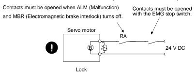
Refer to section 4.11.3 when wiring for the circuit configuration.
