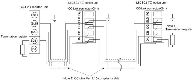
Note 1. Use the termination resistor supplied with the programmable PC or PLC...etc. The resistance of the termination resistor depends on the cable used.
