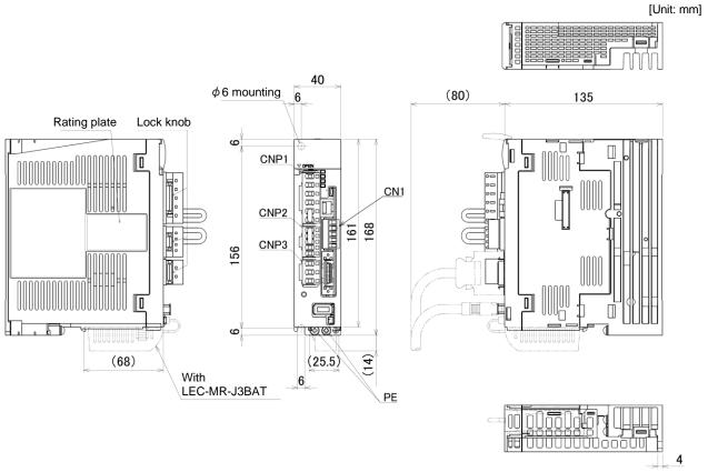
Note. This data applies to the 3-phase or 1-phase 200 to 230VAC power supply models.
