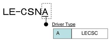
\*LE-CSNA is 10126-3000PE(Connector)/10326-52F0-008 (Shell kit) of Sumitomo 3M Limited or equivalent goods.
