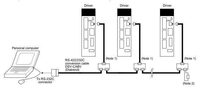
Note 1. The BMJ-8 (Hakko Electric Machine Works) is recommended as the branch connector.
