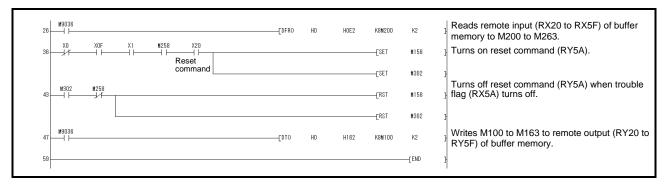
(b) Deactivate the alarm of the driver of station 2 using the instruction code.
