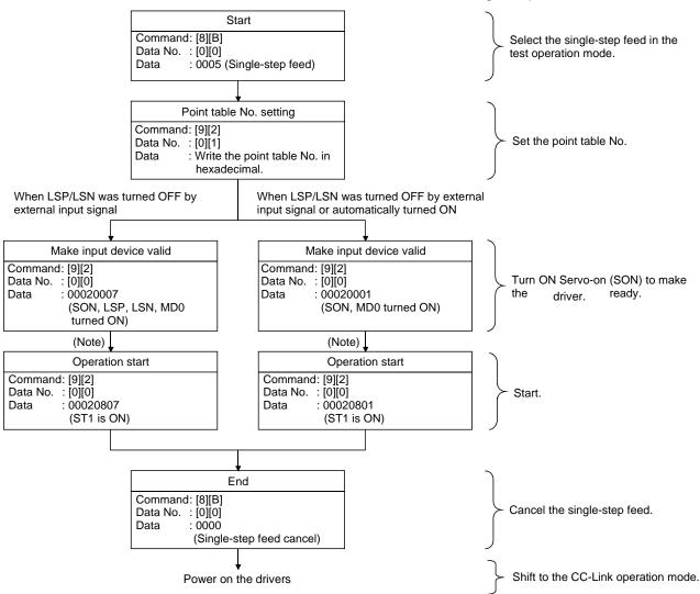
Note. Start operation after home position return completion (ZP) is confirmed. Refer to 17th bit of the data read with command [1][2] and data No.[8][0].
