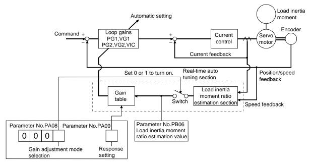
When a servo motor is accelerated/decelerated, the load inertia moment ratio estimation section always estimates the load inertia moment ratio from the current and speed of the servo motor. The results of estimation are written to parameter No.PB06 (the ratio of load inertia moment to servo motor). These results can be confirmed on the status display screen of the set up software (MR Configurator2<sup>TM</sup>) section.
