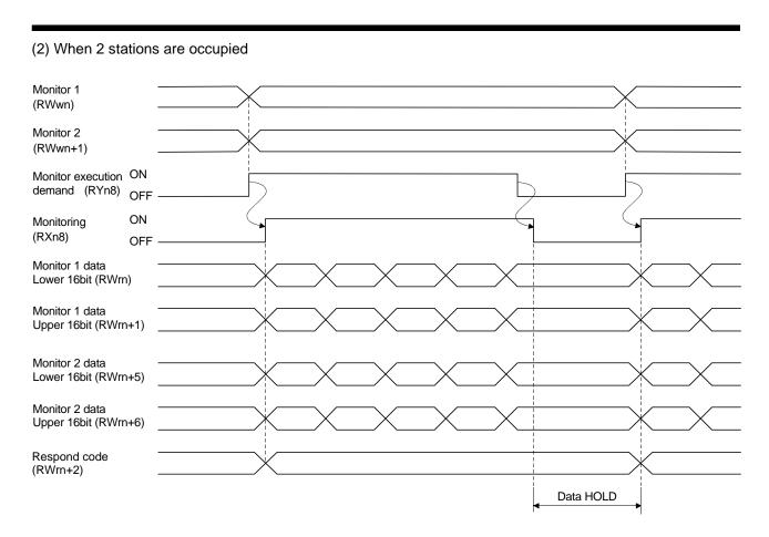
Set the monitor codes (0000 to 001D) (refer to section 3.5.3) to Monitor 1 (RWwn) and Monitor 2 (RWwn+1) and turn Monitor output execution demand (RYn8) to ON. Turning Monitor execution demand (RYn8) to ON sets the next data. 32-bit data are all divided into the upper 16 bits and lower 16 bits, and set to the remote register. Data are all hexadecimal numbers. At this time, Monitoring (RXn8) turns to ON at the same time.
