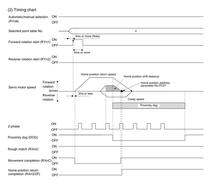
Note. Configure a sequence that changes the point table selection earlier, considering the delay time of CC-Link communication.
