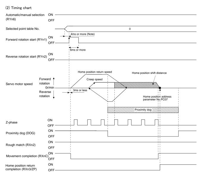
Note. Configure a sequence that changes the point table selection earlier, considering the delay time of CC-Link communication.
