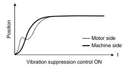
When the advanced vibration suppression control (vibration suppression control tuning mode parameter No.PB02) is executed, the vibration frequency at machine side can automatically be estimated to suppress machine side vibration.
