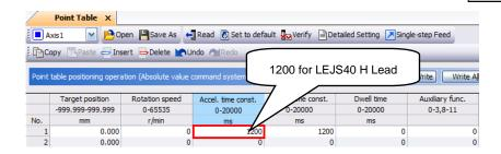
\*4. Use the acceleration time constant of Point table No.1 as the acceleration time constant (msec) of Home position return. Set the recommended value in the above figure. Refer to "LECSC2-T
