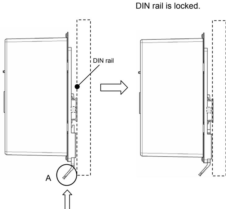
Hook the controller on the DIN rail and press the lever of section A in the arrow direction to lock it.
