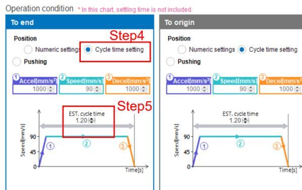
Step5: The theoretical cycle time setting can be changed. However, it cannot be set shorter than the theoretical time when the cycle time setting is enabled.
