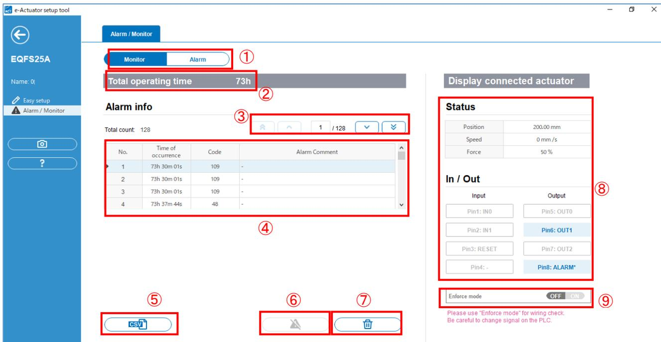
①Switching tabs : "Monitor" : Current product status can be checked, alarm history can be checked, and output signals can be forced.
