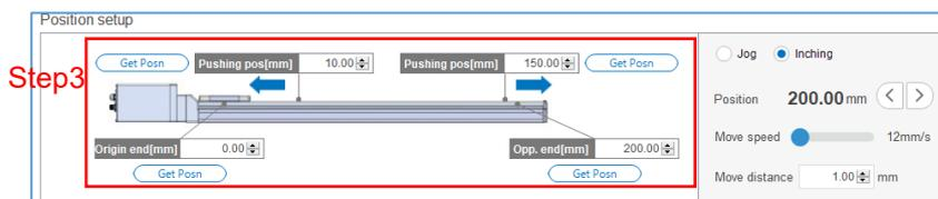
Step3: In the position setup, set the origin end, the opposite end, and the start position of the pushing position.
