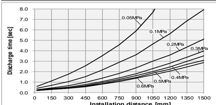
**5-2. Static neutralization range (Discharge time of 1000V→100V)**
