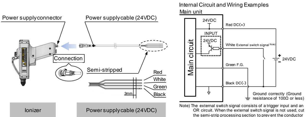
Note) The external switch signal consists of a trigger input and an OR circuit. When the external switch signal is not used, cut the semi-strip processing section to prevent the conductor from making contact.
