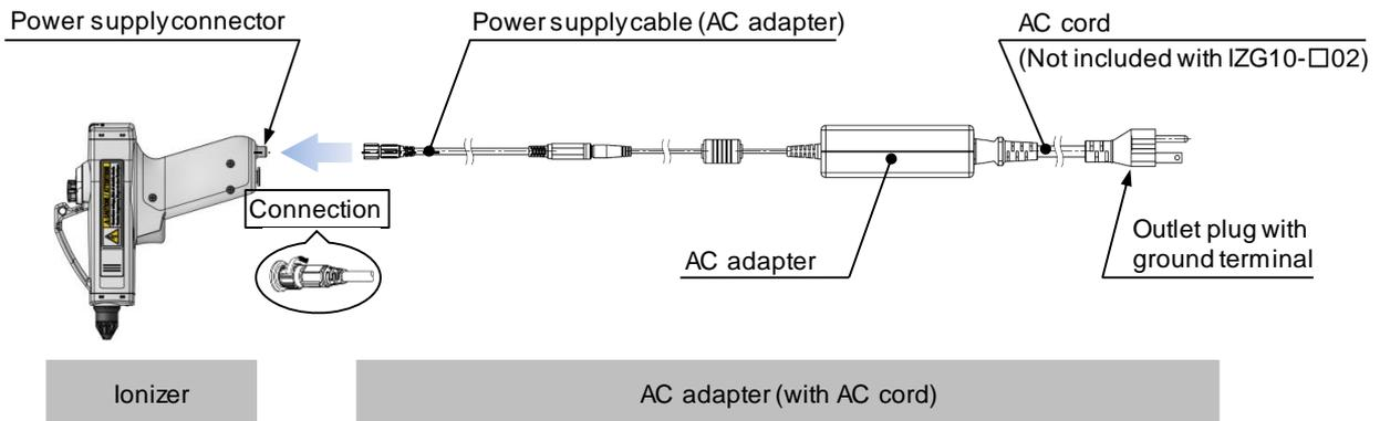
Note) The rated voltage of the AC cord supplied with IZG10-□01 is 125V, and the plug is JIS C8303 type B, which is for Japanese domestic use. If the product is used in an area other than rated voltage (220 or 240VAC), select IZG10-□02 without AC power cord and prepare an AC cord with ground terminal inlet IEC60320-C13 adapted to the power supply voltage.
