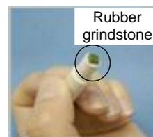
Use if dirt cannot be removed with felt.
