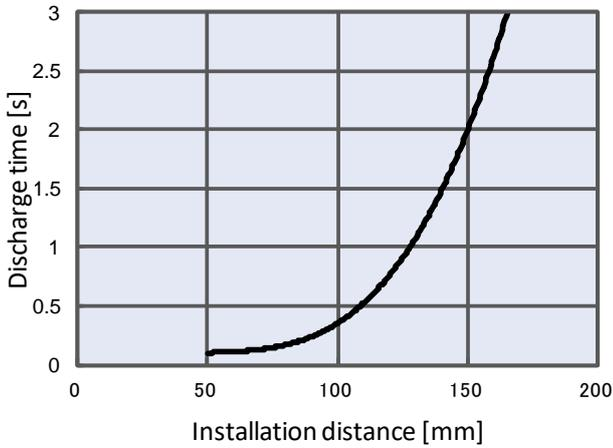
2) With High speed static neutralization cartridge
