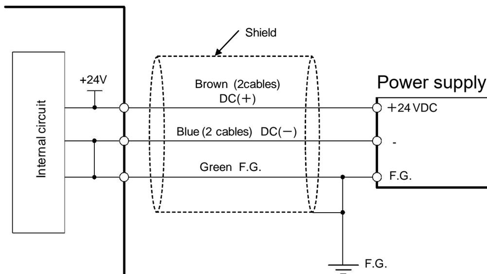
**Make sure to ground the F.G. cable (green) with a resistance of 100 ohms or less. Without grounding, this products and/or power supply may be damage.**
