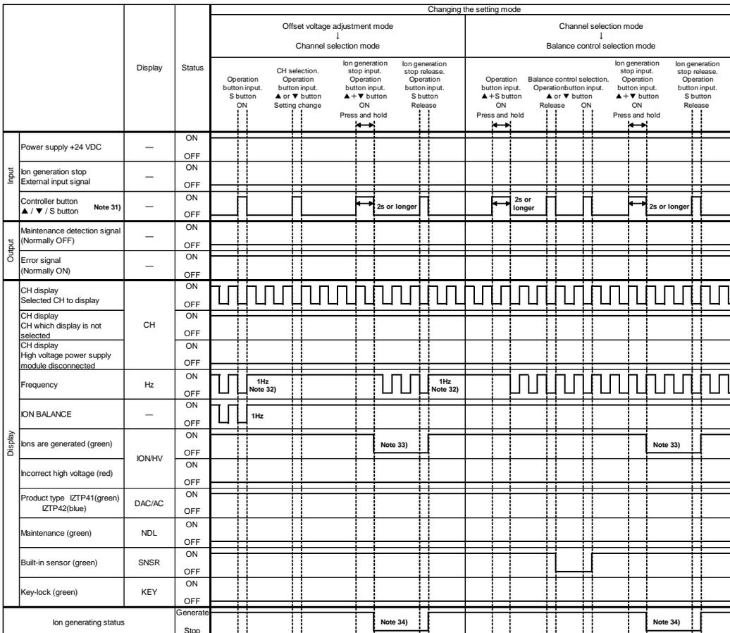
Note 31) Press the controller button once or for 2 seconds or longer to change/set of the setting mode and stop/release the ion generation.
