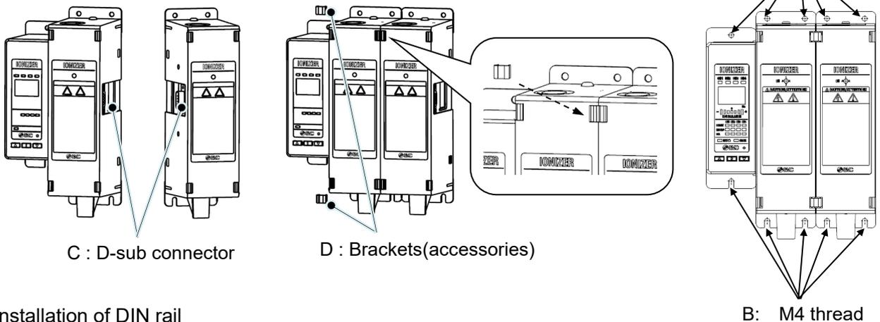
2) Installation of DIN rail
