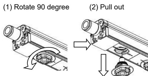
Removal procedure of emitter cartridge
