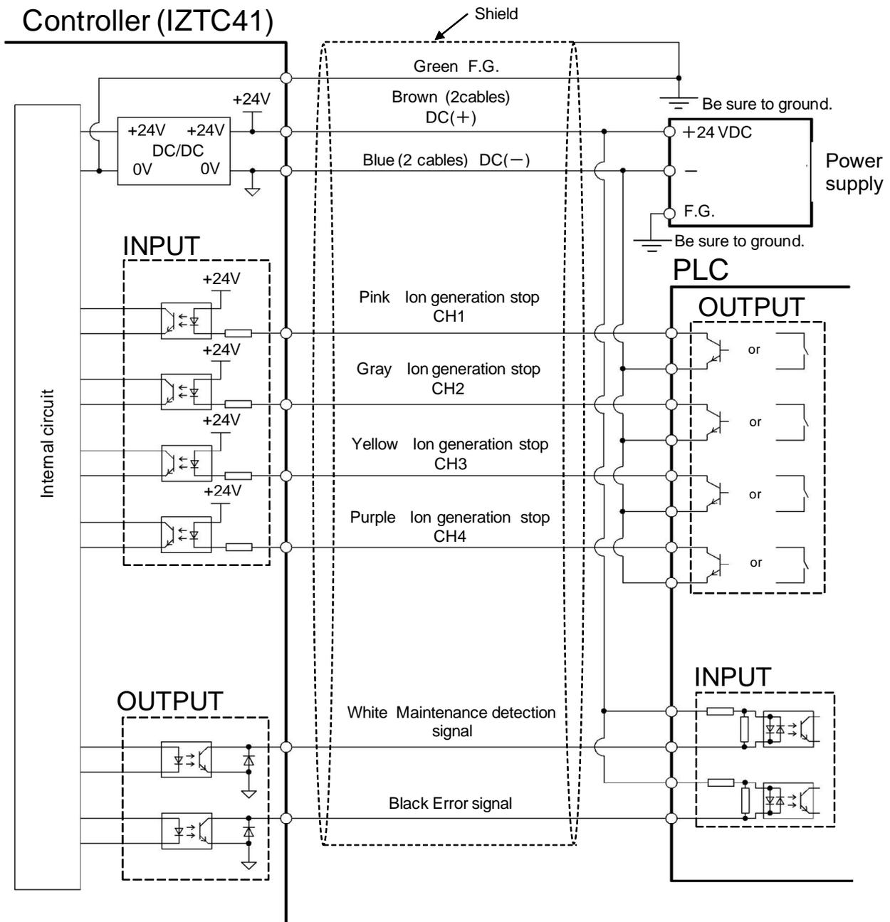
**Make sure to ground the F.G. cable (green) with a resistance of 100 ohms or less. Without grounding, this products and/or power supply may be damaged.**
