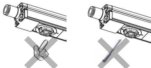
**9) Do not affix any tape or labels to the controller, high voltage power supply module or bar.**
