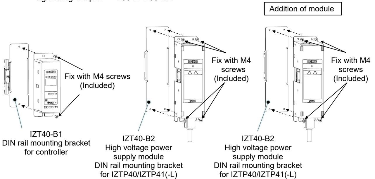
c. Connect the controller and high voltage power supply module
