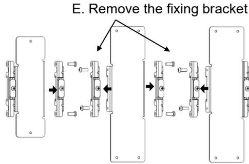
b. Mounting of DIN rail mounting bracket
