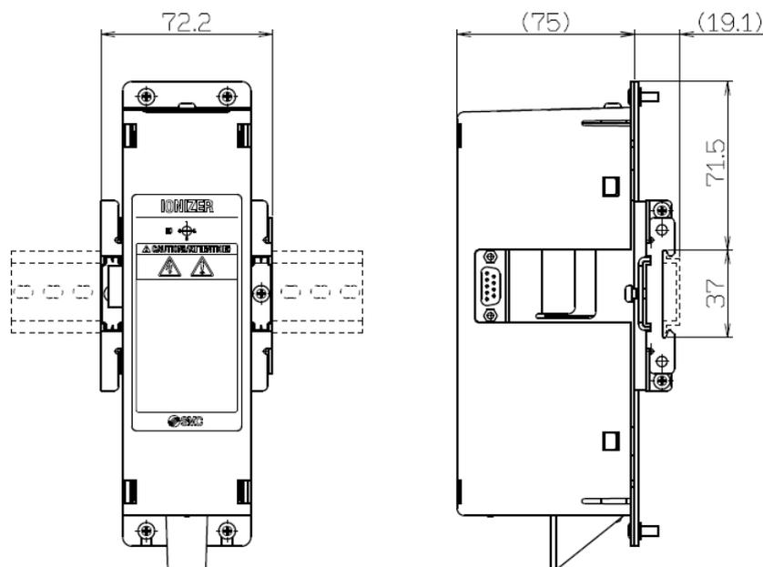
High voltage power supply module IZTP42 (IZT42)
