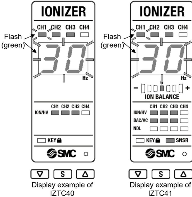
Example of frequency setting mode for CH1.
