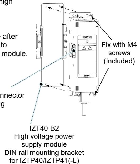
III. When the high voltage power supply module is added directly
