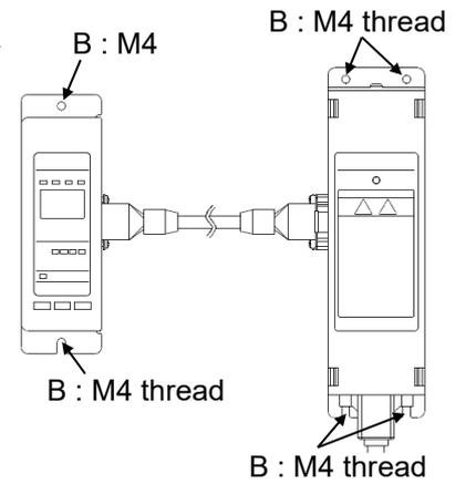
III.Adding a high voltage power supply module
