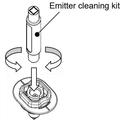
d. When the emitter cartridges are removed for cleaning, remount them to the bar according to the "Mounting procedure of emitter cartridge" shown below. Make sure that the cartridges are securely mounted. If not, the cartridges may become dislodged when compressed air is supplied to the ionizer.
