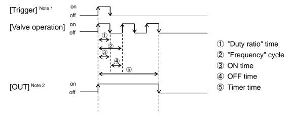
Example 4) Trigger one shot input mode: the trigger starts and stops the valve operation.
