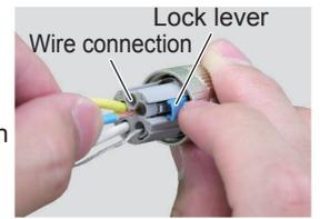
When the wire is inserted, close the lock lever back to its original position. For CC-Link and DeviceNet®, insert the shield \*1 into terminal No.1 (grey). In case of the wire with a ferrule, insert directly. The color coding is previously printed on the connector according to the wire color. (Refer to the connection on the left side.)
