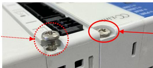
If the unit connecting screw is correctly tightened, the unit connecting screw will be in the lowered position.
