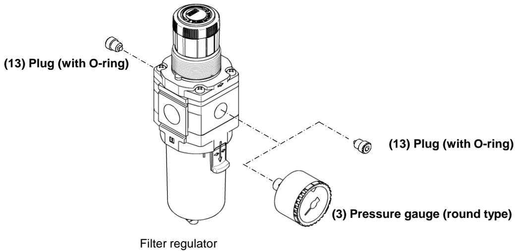
12-3. Disassembly Drawing of the Pressure Gauge Port
