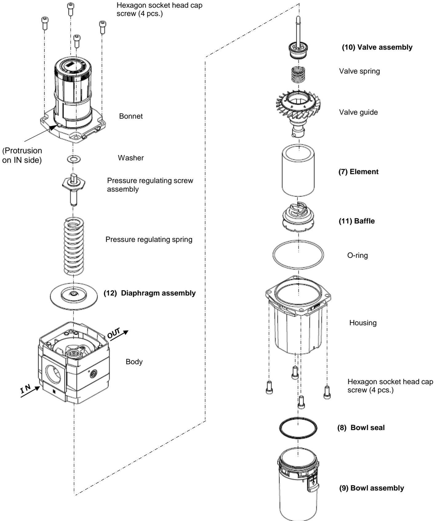
12-2. Disassembly Drawing of the Pressure Gauge Port
