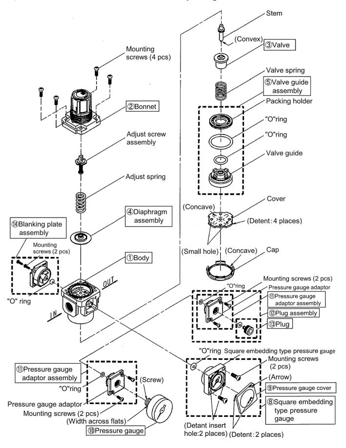
Note) It is possible to mount ®Square embedding type pressure gauge or ①Pressure gauge adaptor assembly or ②Plug assembly instead of ④Blanking plate assembly.
