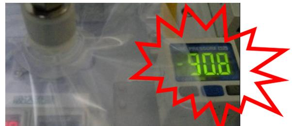
**Suction pad for thin workpiece -90.8kPa**
